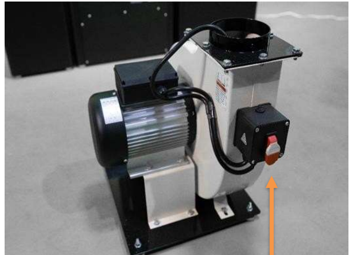
Exhaust Blower switch
